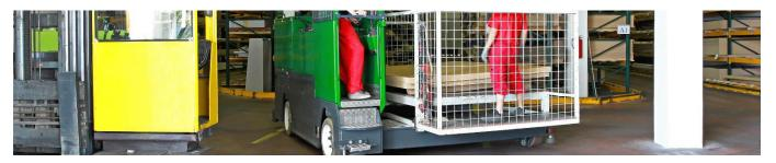
A forklift work platform is a unit or cage that is supported on a lift truck. The use of a platform allows employees to work at heights or in difficult-to-reach places. If not operated properly, they can cause serious injury and even death. To reduce the risk, workers should follow these safety tips and warnings
